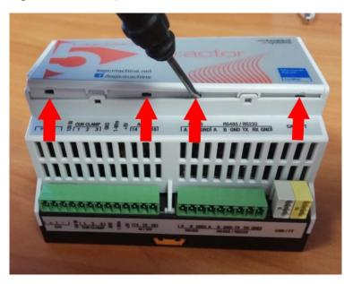
2) Open MicroSIM holder by moving down the top part and lifting up
