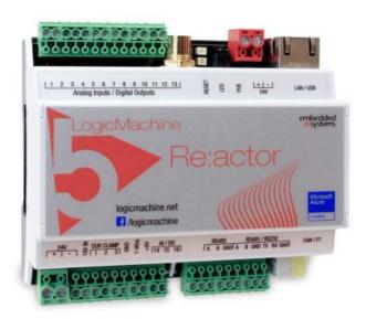
integration with cloud/web services, 3<sup>rd</sup> party devices. Via applying custom scripts LM can simultaneously act as thermostat, security panel, lighting controller, etc. LogicMachine application store and external app development possibility allows to extend device functionality and adjust to a specific market segment.
