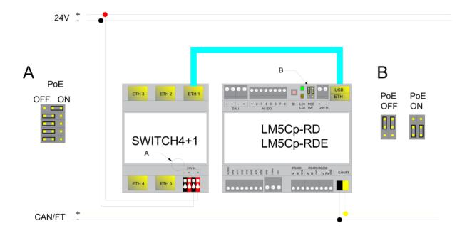
Please note that there are two PoE types of PoE switches/adapters – passive and active (802.3af). In passive mode 4 Ethernet cable wires are used for data and 4 are used for power. In active PoE mode data and power goes together.
